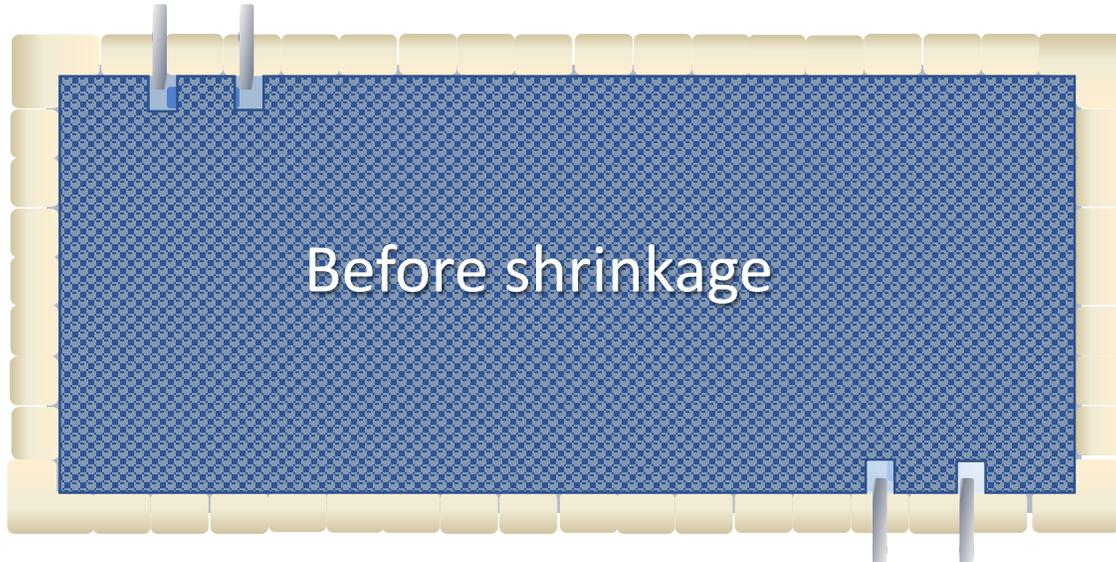
Shrinkage can be most problematic when cutting around ladders and fixed features within the pool.
