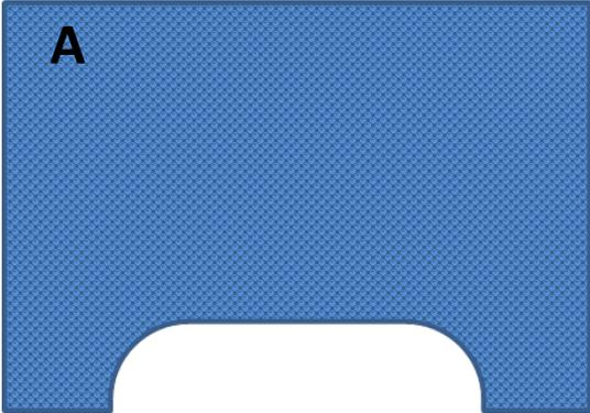
**Image A:** The Rounded cut prevents tear propagation should the material become caught on the ladder while being reeled on or off the pool.
