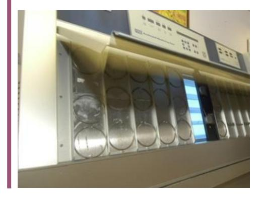
To ensure the product's lifespan, Plastipack internally tests accelerated weathering samples subjected to a high chlorine solutions.
