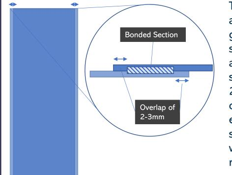
The upper and lower guides should be adjusted such that a 2-3mm overlap exists each side of the welded region.
