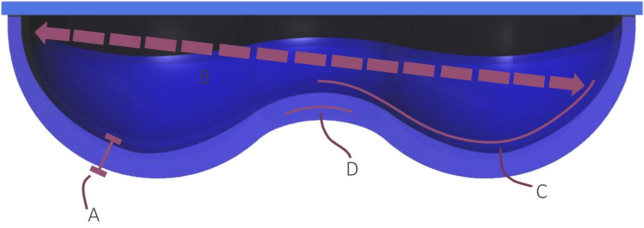
$\begin{array}{l} A-50\% \mbox{ thicker at its thinnest point to resist chemical attack.} \\ B-\mbox{ Larger bubble profile provides increased room for expansion.} \\ C-\mbox{ Smooth curved structure reduces stresses within the material.} \\ D-\mbox{ Structural arch resists bubble collapse.} \end{array}$
